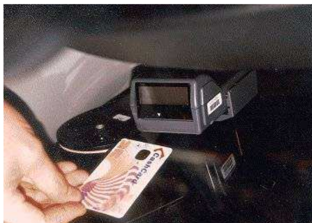
Figure 12 Smart Card OBU for the Electronic Road Pricing Scheme in Singapore 9
