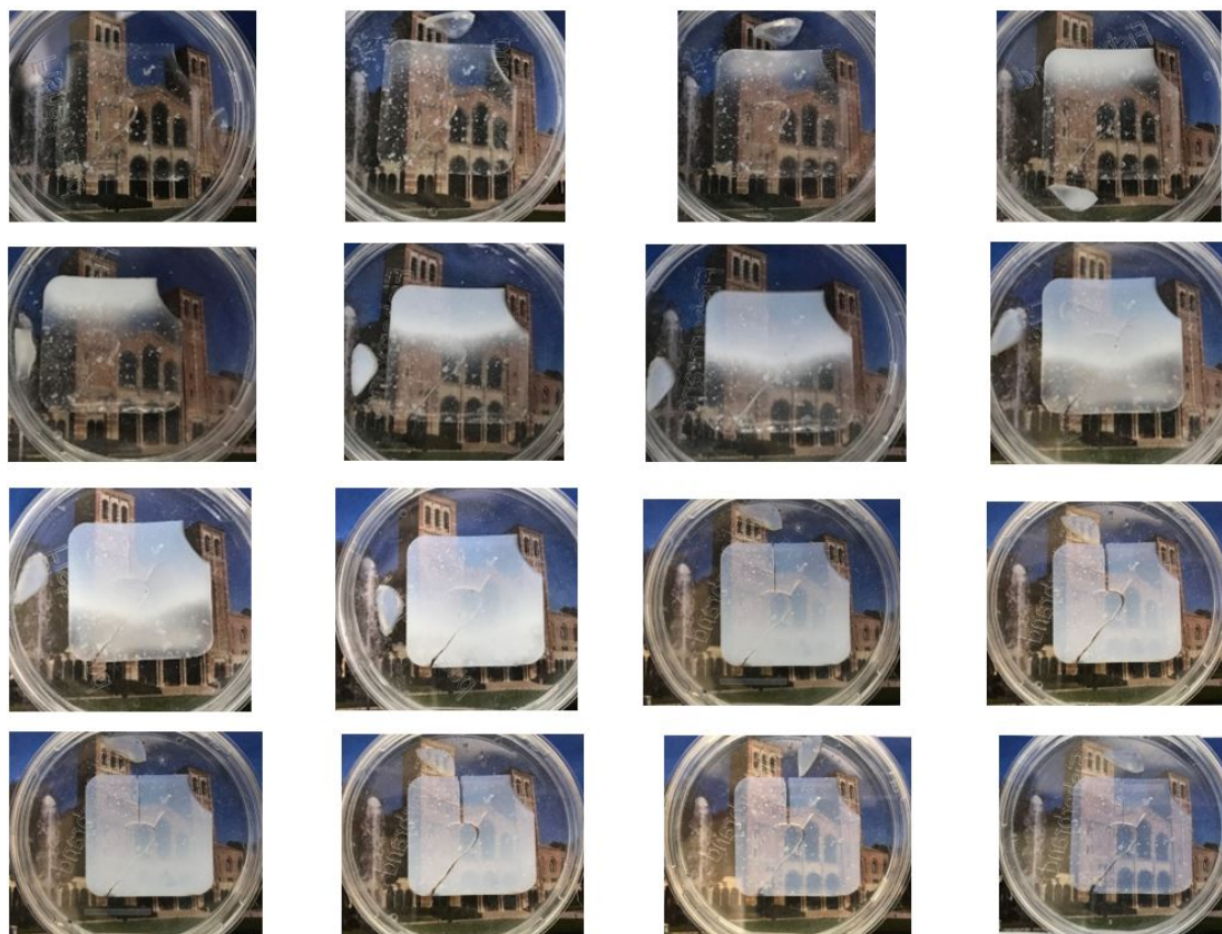
Figure D.2: Photographs of a nanoparticle-based mesoporous silica monolith drying from water in a covered dish. The monolith was photographed on an image of UCLA Royce Hall [22] (modified and redistributed with permission from Ref. [23] Copyright Prayitno).
