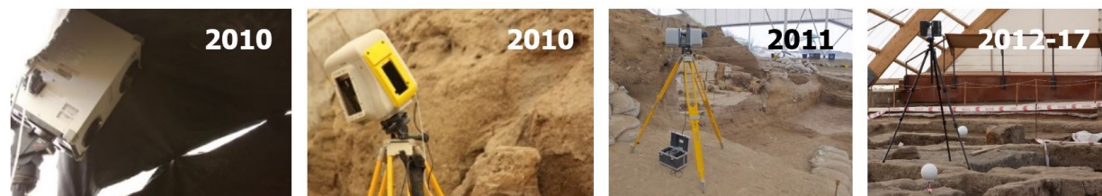
Figure 7.5. Terrestrial laser scanning units used at Çatalhöyük between 2010 and 2015, from left to right: Minolta Vivid 910; Trimble GX; Trimble FX; FARO Focus 3D S120.
