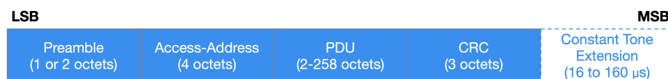
Figure 11. Structure of a Bluetooth 5.1 packet with the duration and position of the CTE. Associated apps add CTE to conventional packets, while those without a connection use an advertizing packet.
