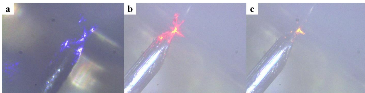
Figure 1.6. Photograph taken with a digital camera, showing the relative position between the scanning tunneling microscope probe tip and (a) 405 nm, (b) 633 nm, and (c) 780 nm laser illuminations spot. We use 36^\circ as the incident angle for all three lasers.
