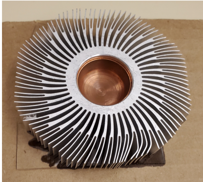
Figure 5.4: Picture of an Intel Corporation heat sink used in these experiments. Multiple identical models were purchased, cooling fans removed, visibly inspected for defects, particularly at the mating surface, then attached to a coil with a TIM.
