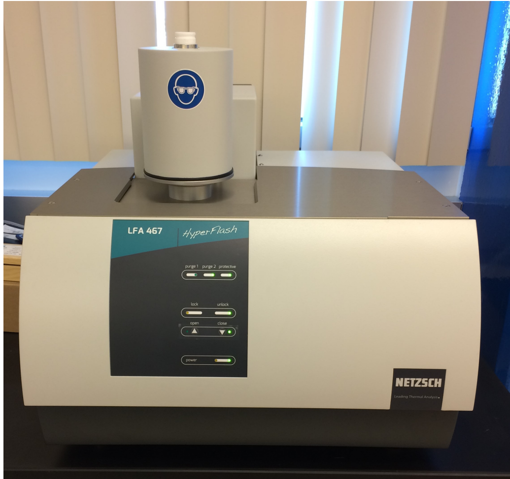
Figure 3.1: LFA 467 HyperFlash equipment by NETZSCH GmbH used in this study.
