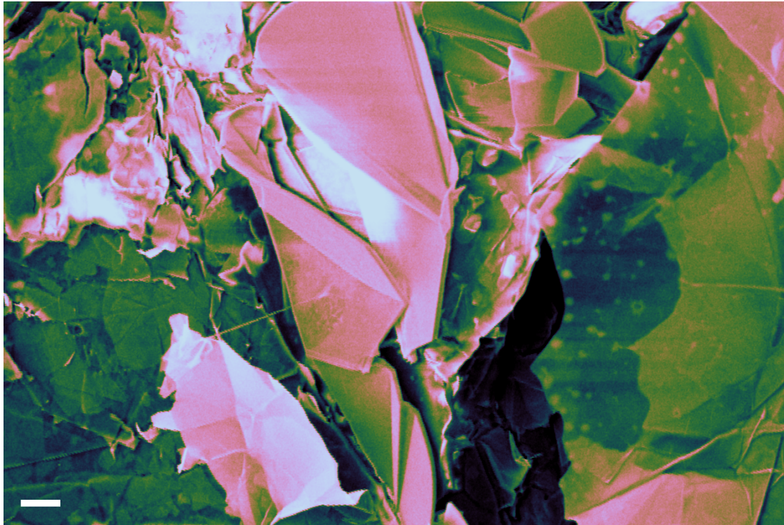
Figure 4.2: Pseudo-colored SEM of a 20 wt. % graphene and 20 wt. % h -BN sample with a 1 micron scale bar. Reprinted with permission from the publication J. S. Lewis, Z. Barani, A. S. Magana, F. Kargar, and A. A. Balandin, “Thermal and electrical conductivity control in hybrid composites with graphene and boron nitride fillers” Materials Research Express , vol. 6, no. 8, p. 085325, May 2019. Copyright © Institute of Physics.
