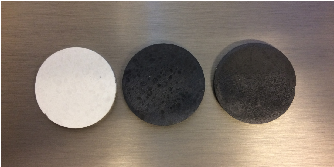
Figure 2.7: Three samples of representative geometries. Hybrid composite samples pictured from left to right: 00 vol. % of graphene and 43.6 vol. % of h -BN, 21.8 vol. % graphene and 21.8 vol. % of h -BN, and 43.6 vol. % of graphene and 00 vol. % of h -BN. The pictured composite samples are at end-of-process and thus have some blemishes that wouldn't normally be as striking.
