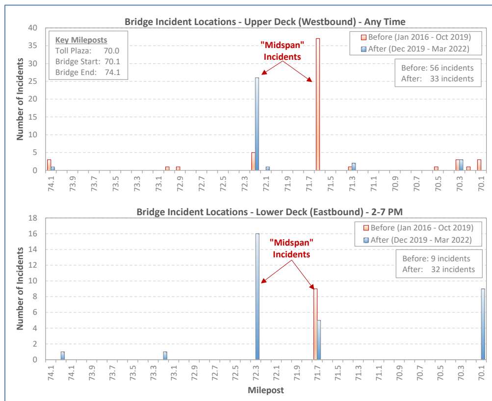
Figure 11-1: Location of Bridge Incidents – Before/After
