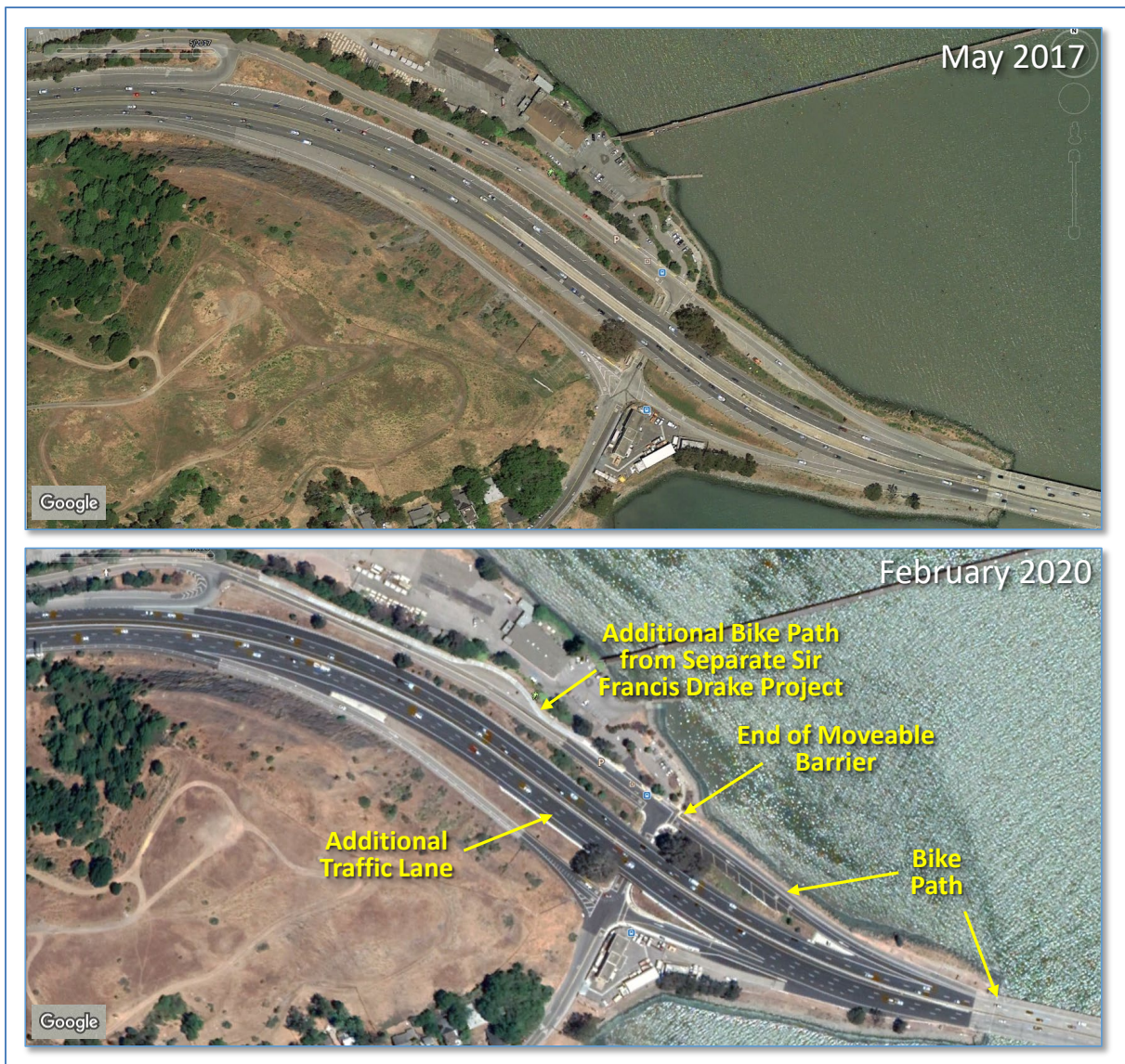
Figure 2-19: Modifications of Marin County Approach
