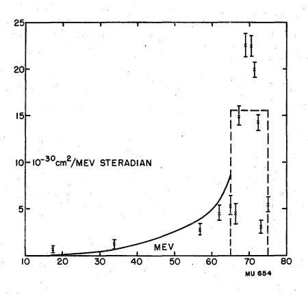
Fig. 10. Differential cross section for meson production at 340 Mev. The definitions and symbols are the same as Fig. 9, except that the transition operator is assumed to be of the form given in Eq. 17, i.e. linearly dependent on meson momentum and leading to a mixture of singlet and triplet spin states.
