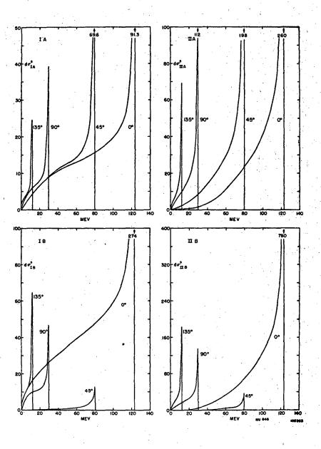
Fig. 4. Differential cross section for meson production. The incident energy is 400 MeV, the final nucleons are assumed to be in a singlet spin state.
