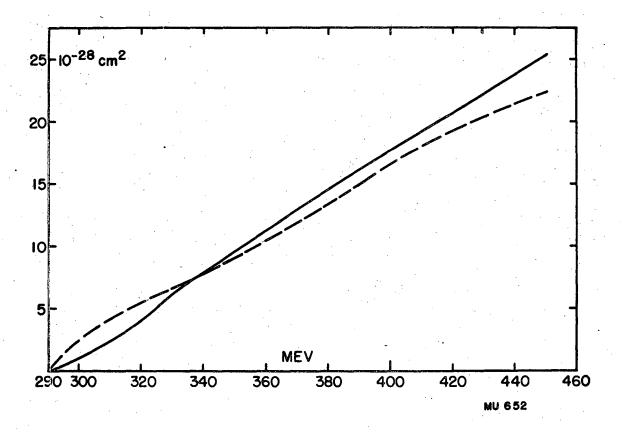
Fig. 7. Variation of the total cross section for meson production with the energy of the incident nucleon. The transition operator  $R_0$  (see Eq. 3) is assumed to be independent of meson momentum. The cross sections are arbitrarily normalized to  $8 \times 10^{-28}$  cm<sup>2</sup> at 340 Mev. The solid curve is for a final nucleon singlet state, the dashed curve is for a final nucleon triplet state and includes the possibility of deuteron formation.
