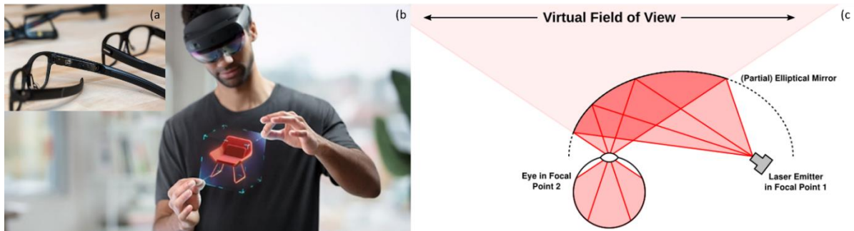
Figure 1-6 Shows an image of Intel's Vaunt smart glasses (a) and Microsoft's HoloLens 2 (b) that used VCSELs and EELDs as illumination sources, respectively 39,40 . A schematic showing the laser light being projected on the retina is shown in (c) 41 .
