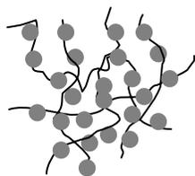
Figure 2. Schematic illustration of non-woven media with sorbent granules bonded to the fibers.
