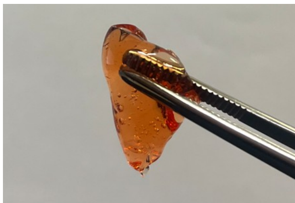
Figure 4.3 - The viscoelastic flow behavior of the PEG-based hydrogel over time. Left: The freshly shaped hydrogel retaining a defined three-dimensional form immediately after transfer from the tube to the dish. Right: The same hydrogel after 1 hour, demonstrating significant fluid-like flow and flattening into a thin, uniform disc-like layer under gravitational force.
