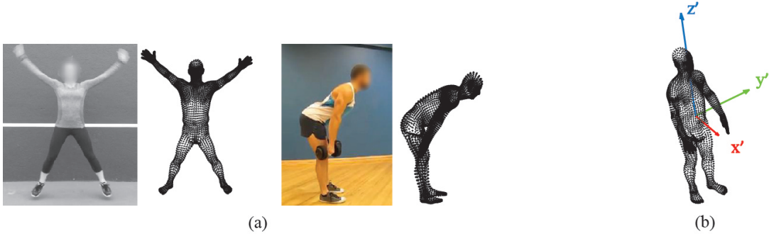
Figure 4.2: (a) Sample reconstructed 3D human mesh from a snapshot of (left) a person doing jumping jacks and (right) a person doing stiff-leg deadlifts. (b) The Local Coordinate System (LCS), defined with respect to the human body.
