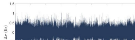
Fig. 3. Eight-hour frequency drift of the stabilized OOL signal relative to the set point of f_{OOL} showing 0.16 Hz rms variance during a typical workday. 1
