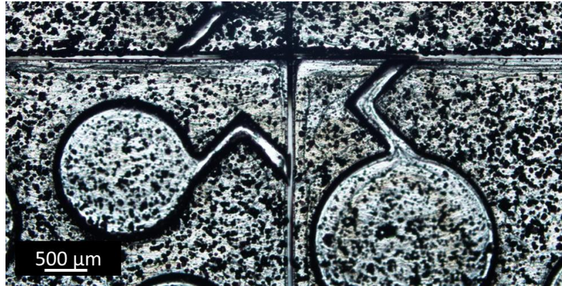
Figure 5.10: Microscope image of a 1 mm diameter and 2 mm diameter circular pit with 50 μm of permalloy and copper electroplated.
