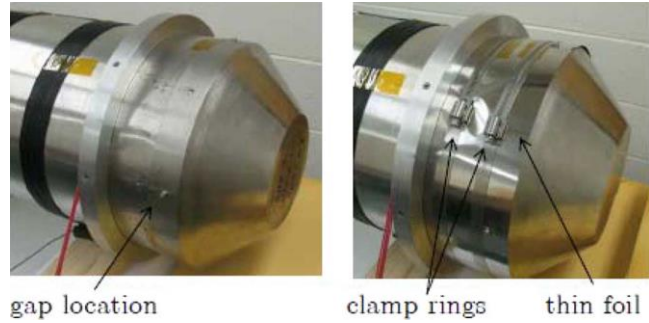
Figure 3.3: Chamber-scale magnetic shield with clamp rings holding a thin foil in place between the cylinder and its endcaps to reduce flux leakage [40].
