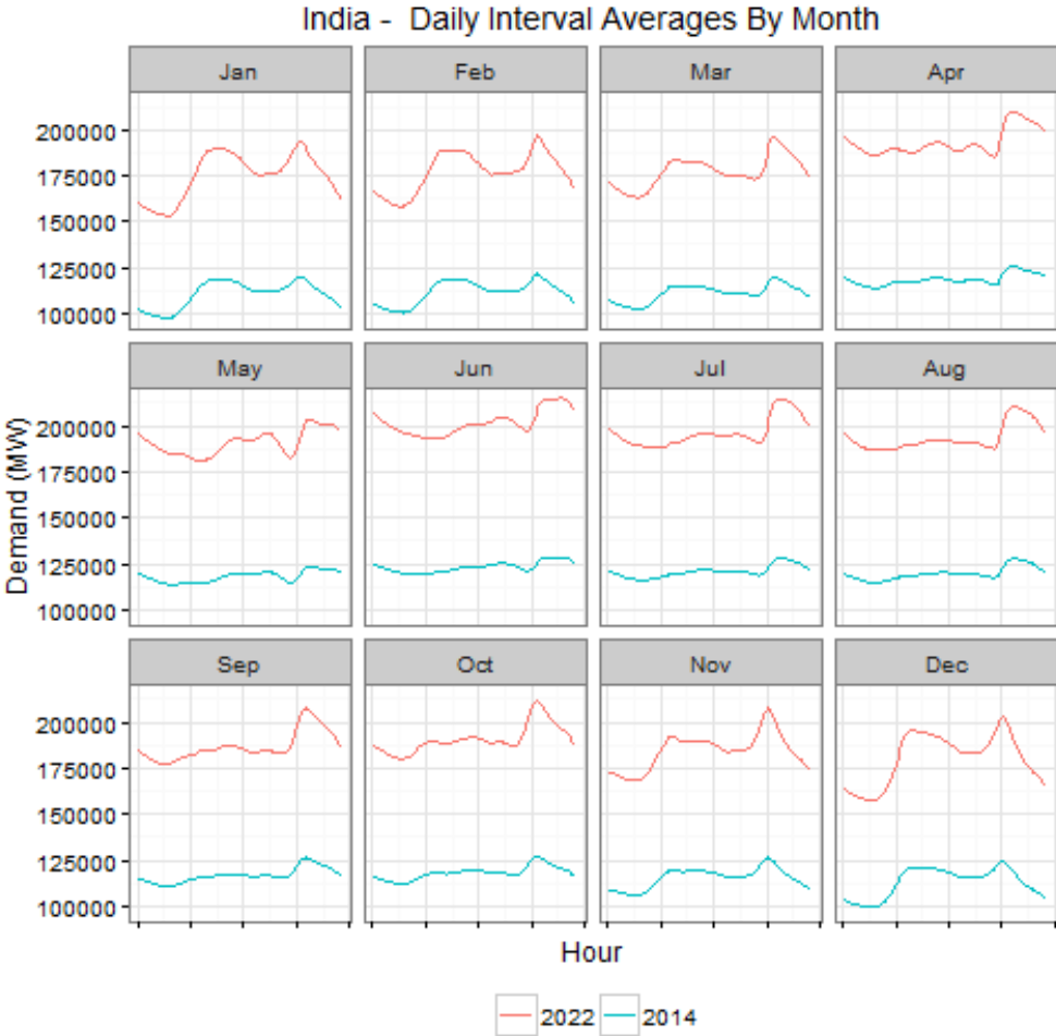
Figure 3.2: Average daily load curves by month for India for 2014 (actuals) and 2022 (forecast).
