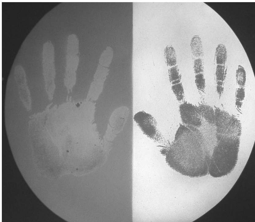
Figure 5-7. Side-by-side comparison of two-step turn-on sensor (left) with fluorescence quenching sensor (right). Tetrabutylammonium nitrite was used as the analyte for the turn-on sensor and TNT was used for the fluorescence quenching sensor.
