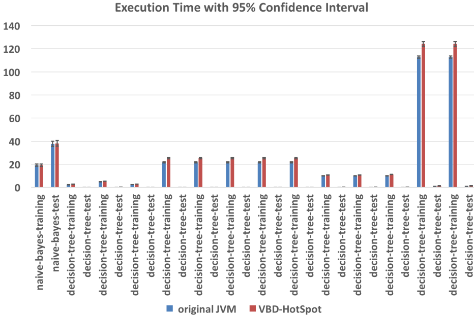
Fig. 7. Average of 10 median execution times in seconds with 95% confidence interval for mllib-tests (part 2 of 4)
