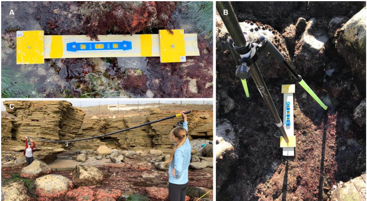
Figure 2: A. A 0.5m scale bar placed in a plot during a field survey. B. The tripod legs of an iG8 RTK GNSS instrument used to collect GPS data of identifiable points in the plot. C. An ~8m pole being held above the survey plot while an attached camera continually captures photos.
