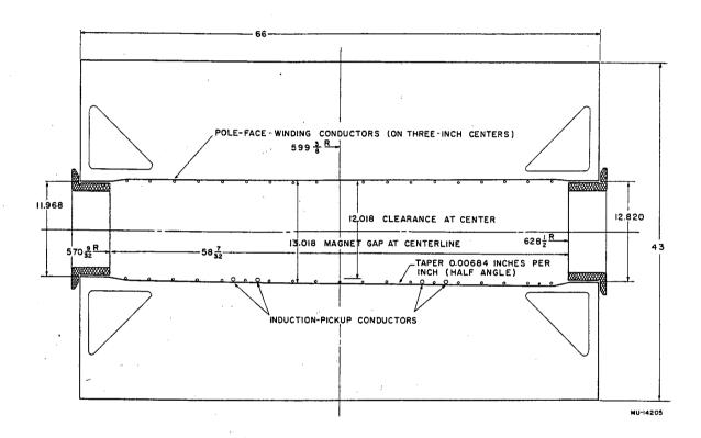
Fig. 11. Dimensions of magnet aperture. All dimensions are in inches.
