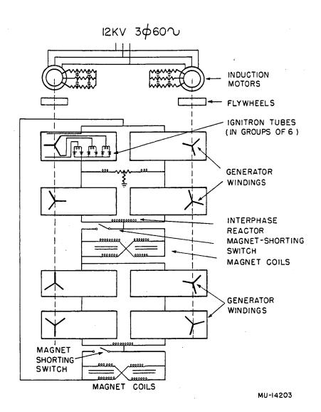
Fig. 13. Bevatron magnet circuit.
