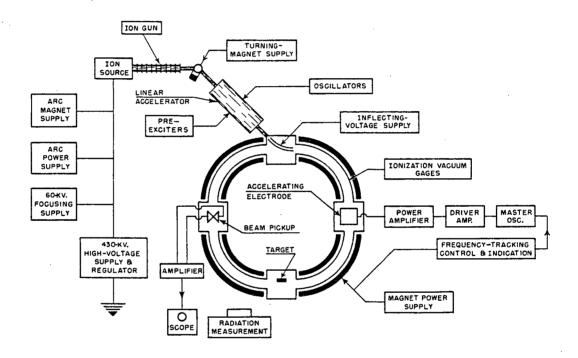
Fig. 1. Diagram of the Bevatron showing the principal electronic elements. Accelerating electrode and beam pickup are shown interchanged from their actual positions.
