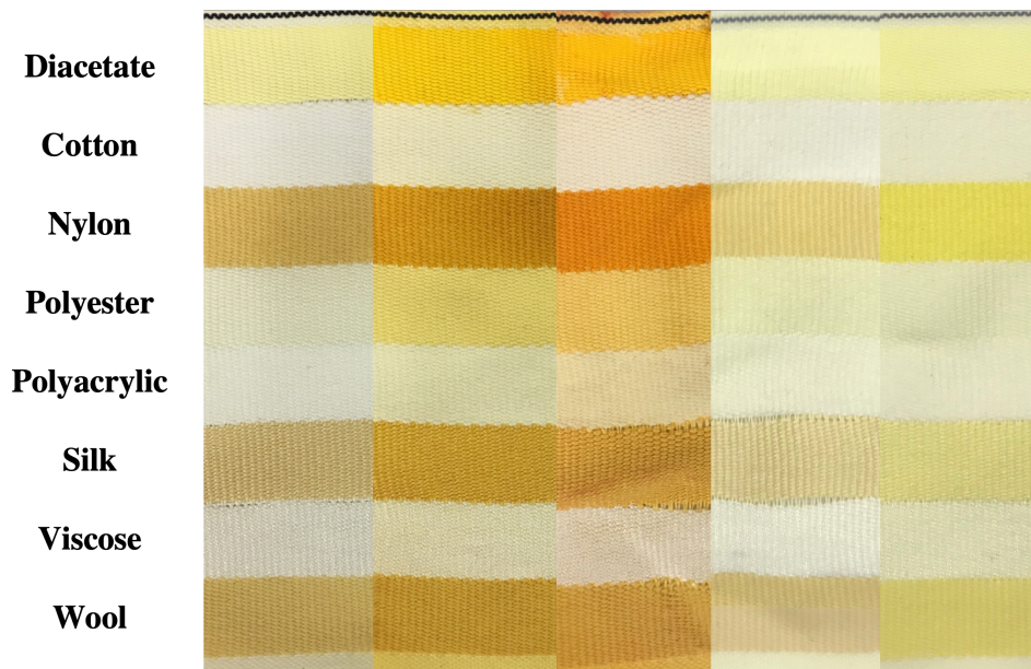
Figure 3.5: Fabrics dyed by CMF derivatives, from left to right: 4 , 5 , 6 , 7 , and 8
