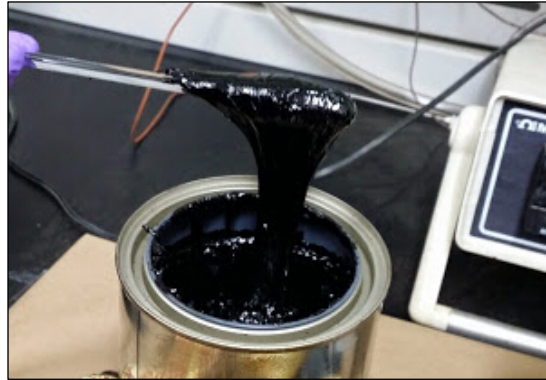
Figure 4.1: Recovered RAS binder after three hours of conditioning at 190°C.
