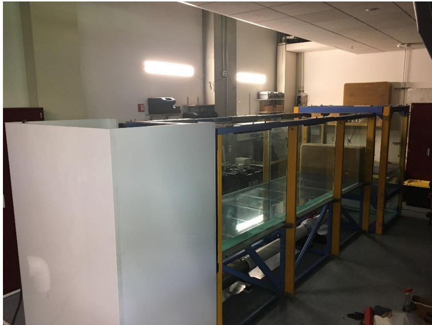
Figure 5.15a: Angled view of filled channel for leak testing.
