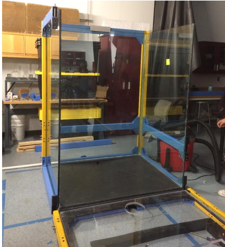
Figure 5.2: Support frame holding together the three tempered glass panels.
