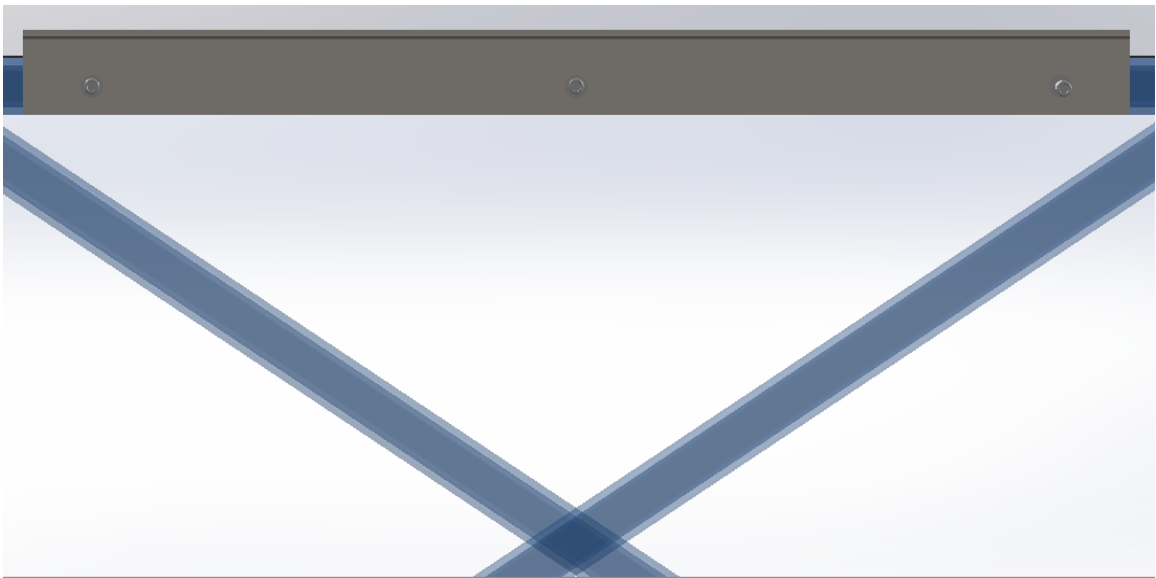
Figure 3.9a: Angle beam to chassis module bolt connection.
