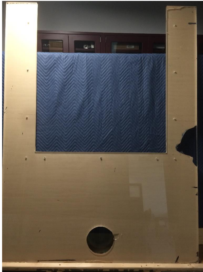
Figure 5.3: Machined Plexiglass front panel.
