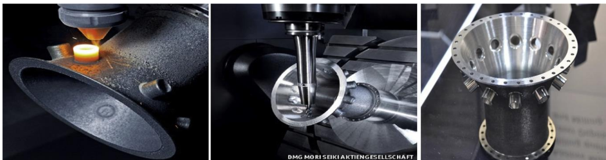
Fig. 1.1: Turbine housing that was created through the DED process. (Left) The part created through multi-axis deposition. (Middle) The part being machined for a better surface finish (Right) The final finished turbine [2].
