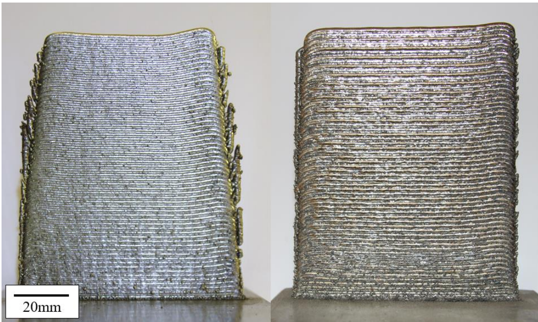
Fig. 4.7: 120-layer thin wall builds with 3 s interlayer dwell (left) without controller and (right) with PID controller
