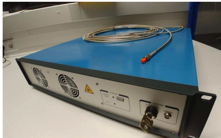
Figure 4.4 The seed oscillator. The system seeds the stretcher with 3.3mW of average power at 50MHz. The system is air cooled with a muffin fan.
