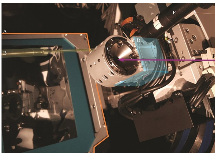
Figure 2. An annotated image of a BX90 diamond anvil cell (DAC) mounted on the Stoe Stadi-Vari diffractometer on beamline 12.2.2, endstation 1. (A) The Research Detectors Inc. (RDI) CMOS 1M detector (Oakland, CA, USA). (B) The beamstop. (C) The BX90 DAC. (D) Motorized DAC alignment XYZ stages. (E) Off-axis sample viewing/alignment camera. (F) Idealized representation of the X-ray beam direction.
