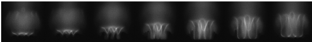
Figure 3.20. Unstable flames on the 7H tip
