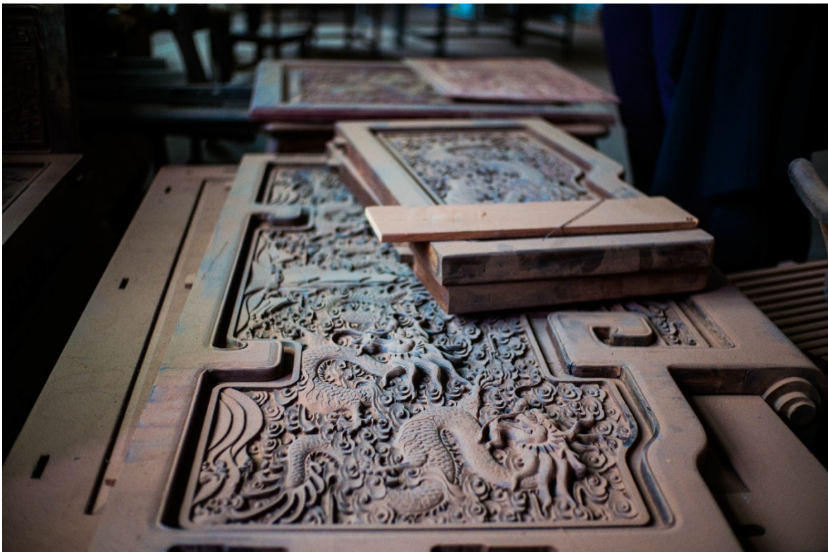
Figure 5. A panel of rosewood decorated with the fortuitous dragon image, carved by machine and to be touched-up by crafters.
