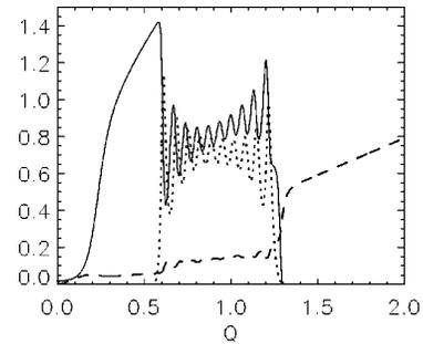
FIG. 1. Evolution of  $\epsilon$  (solid line),  $V_{ZF}$  (dotted line), and  $\mathcal{N}/5$  (dashed line) as a function of input power  $Q = 0.01t$ . Parameter values are  $a_1 = 0.2$ ,  $a_2 = a_3 = 0.7$ ,  $b_1 = 1.5$ ,  $b_2 = b_3 = 1$ ,  $c_1 = 1$ ,  $c_2 = 0.5$ , and  $d = 1$ .
