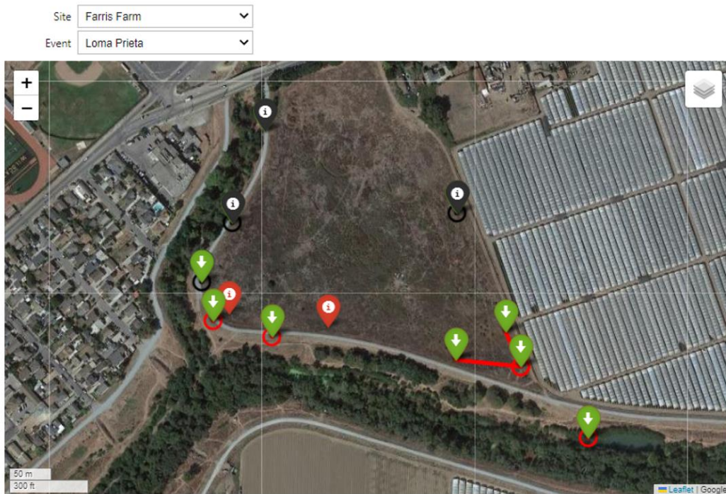
Figure 5-1. A screenshot of the Jupyter notebook that the SMT developed for review of individual case histories. Black markers represent observations of “no manifestation”, red markers represent “yes manifestation”, green markers represent CPTs, red/black lines connect CPTs and observations that the SMT grouped together, and red/black circles indicate a collocated CPT and observation pair (note that the green CPT marker is obscured by the red/black observation marker for collocated CPT/observation pairs).
