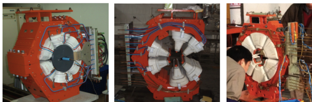
Figure 2: First article magnets of the three different types of magnets. Left: Straight section magnet; Middle: Arc magnet; Right: Special injection straight magnet.
