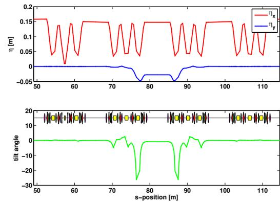
Figure 6: New fs-slicing optics that provides the spatial separation of the energy sliced beam in the new upgrade lattices.
