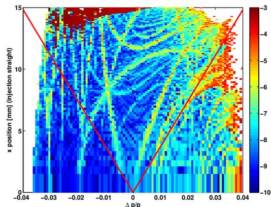
Figure 3: Example of an optimized offenergy frequency map for the baseline lattice (including magnet errors and physical apertures)
