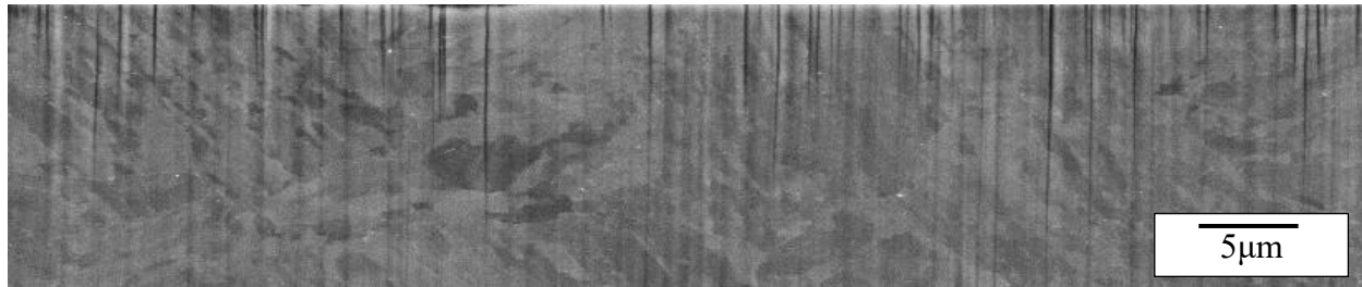
Figure 26. Backscattered electron image of the F82H microstructure showing fine lath martensite
