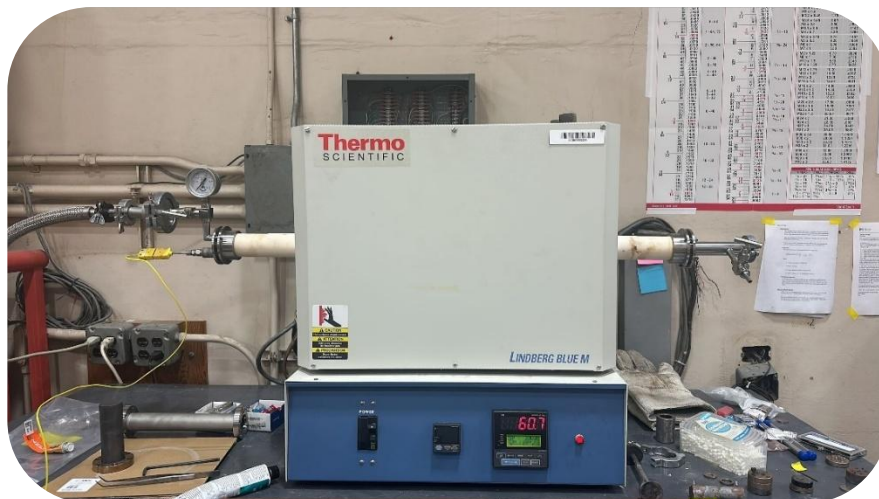
Figure 38. ThermoScientific vacuum tube furnace used for heat treatment
