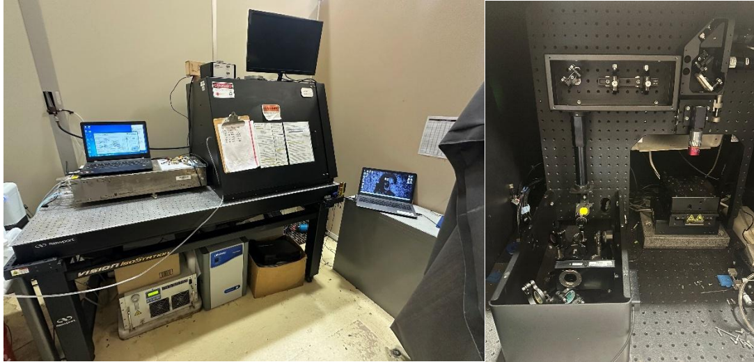
Figure 41. Femtosecond laser setup. Full system with interior view of laser chamber with optics exposed.
