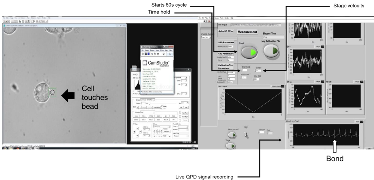
Figure 7.1: A snapshot of the LabView program to conduct Rupture experiment 1: The LabView program “Shreyas_RuptureForce” shows the user interface for performing a rupture experiment. The program has fields to input the File directory to save recorded files, approach and retraction piezo stage velocities, sampling rate and time steps. The QPD signal monitoring window shows the continuous signal generation in cyclic touch and release experiments for user to gauge the signal characteristics and bond formation.
