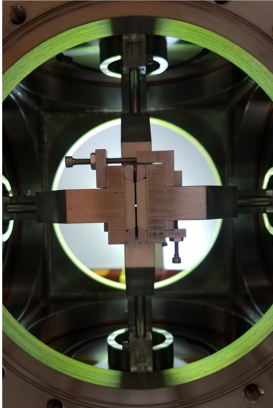
Figure 13.7: The fully closed and aligned experimental structure in the minimum gap configuration. The small square in the center of the image is the beam axis. The dielectric slabs are the lighter components immediately adjacent to the gap and retained by the wedges of aluminum holding them to the strongbacks. The visible screw and nut are the hard-stop system with the screw impacting the angle bracket on the opposing strongback to set the minimum gap.
