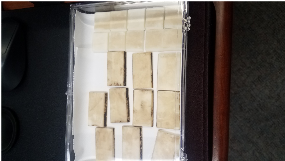
Figure 13.9: The alumina slabs immediately after the machining process. The black substance and staining is from the blocking material used to secure the slabs during work.
