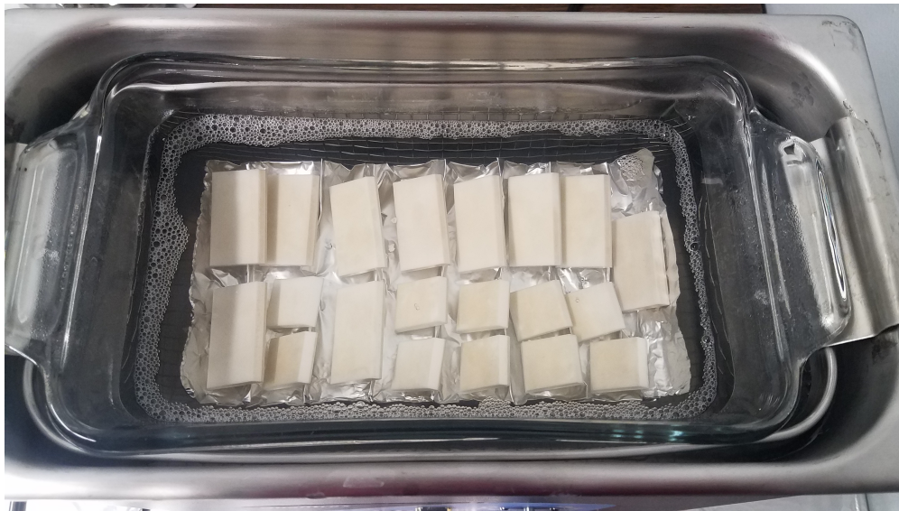
Figure 13.10: The alumina slabs during the cleaning process. In the image they are depicted undergoing an ultrasonic bath. The aluminum foil is used as a cushion to prevent contact between the slabs and the tub wall. It is also folded to prevent contact between the slabs themselves.
