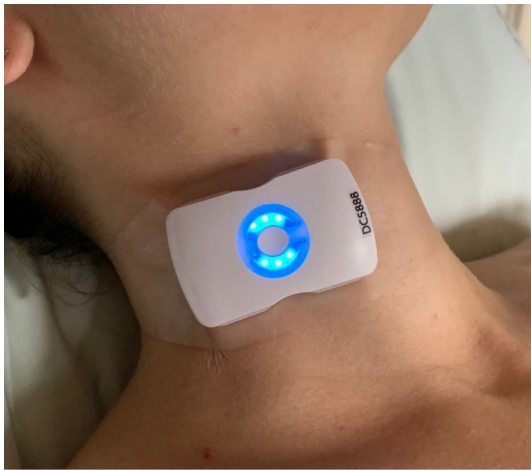
Fig. 1 Picture of wireless, wearable Doppler ultrasound device
