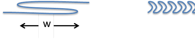
Figure 7.1: The trilayer folding morphologies discussed in the text: left, S-fold of width w ; right, crinkle fold.
