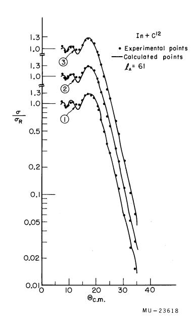
Fig. 18. Angular distribution of  $C^{12}$  ions elastically scattered from In at  $E_{lab} = 124.5$  Mev. The dots are the measured cross sections and the solid line is the calculated cross section with the following McIntyre model parameters.
