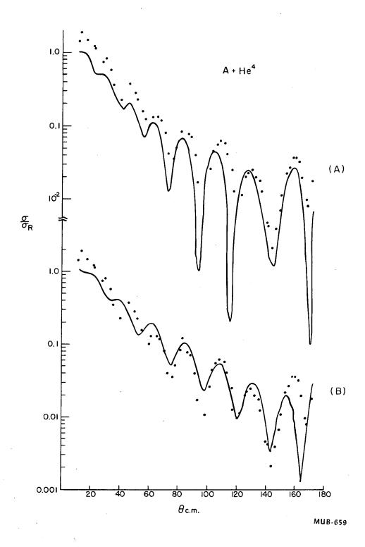
Fig. 25. (A) The solid line is the optical-model fit to the elastic scattering of a's from A (Ref. 55). Parameters are  $V_0 = 100$ ,  $W_0 = -15$ ,  $R = 1.17A^{1/3} + 1.36$ , d = 0.6. The points give the experimental values.
