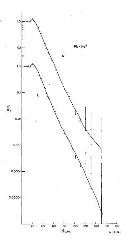
Fig. 27. (A) Same as 25A for a's scattered from Pb (Ref. 55). The parameters are  $V_0$  = -25,  $W_0$  = -15, R = 1.13A<sup>1</sup>/3+2.0 d = 0.6. (B) Same as 25B. The parameters are  $\ell_A$  = 21,  $\Delta\ell_A$  = 1.3,  $\delta$  = 0.2,  $\ell_\delta$  = 23,  $\Delta\ell_\delta$  = 1.4.
