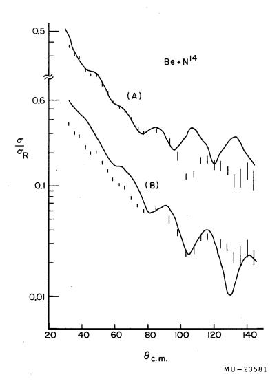
Fig. 28. (A) Same as 25A for N<sup>14</sup> scattered from Be (Ref. 52). The parameters are  $V_0 = -50$ ,  $W_0 = -16$ ,  $R = 1.23A^{1/3}$ , b = 1.125, d = 0.65.
