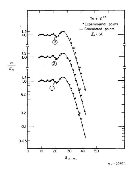
Fig. 15. Angular distributions of  $C^{12}$  ions elastically scattered from Ta at  $E_{lab} = 124.5$  Mev. The dots are the measured cross sections and the solid line is the calculated cross section with the following McIntyre model parameters.
