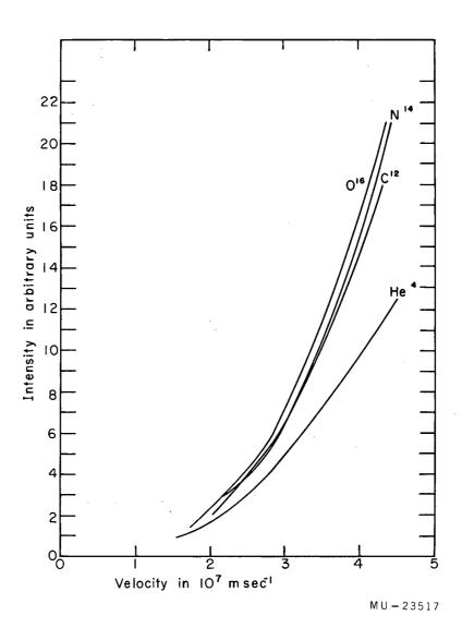
Fig. 9. Response of CsI as a function of velocity.
