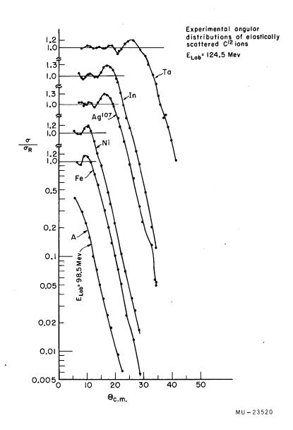
Fig. 14. Experimental angular distribution of  $C^{12}$  ions elastically scattered from A, Fe, Ni, Ag107, In, and Ta.
