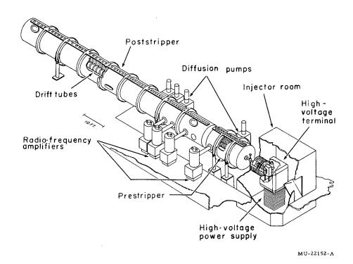
Fig. 5. Schematic view of the Hilac (from Ref. 15).
