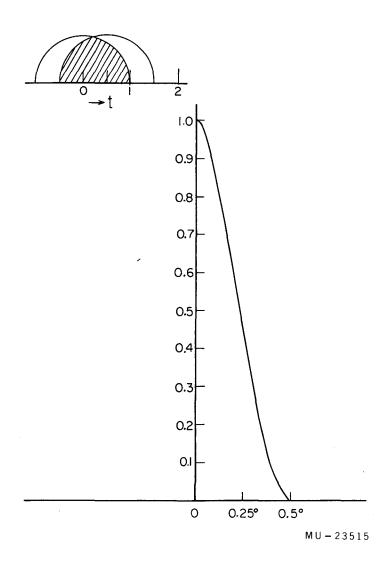
Fig. 13. Distribution of intensity over the angle, calculated by "folding" the two distributions in the insert.
