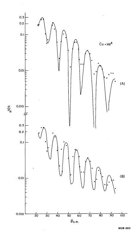
Fig. 26. (A) Same as 25(A) for a's scattered from Cu (Ref. 55), The parameters are  $V_0 = -49.3$ ,  $W_0 = -11$ ,  $R = 1.14A^{1/3} + 2.24$ , d = 0.5. (B) Same as 25B (Ref. 55). The parameters are  $\ell_A = 17$ ,  $\Delta \ell_A = 0.8$ ,  $\delta = 0.7$ ,  $\ell_{\delta} = 17$ ,  $\Delta \ell_{\delta} = 1.0$ .
