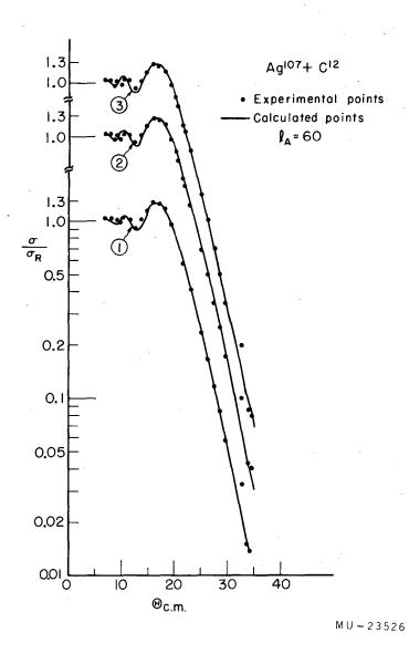
Fig. 20. Angular distribution of  $C^{12}$  ions elastically scattered from  $Ag^{107}$  at  $E_{lab}=124.5$  Mev. The dots are the measured cross sections and the solid line is the calculated cross section with the following McIntyre model parameters.
