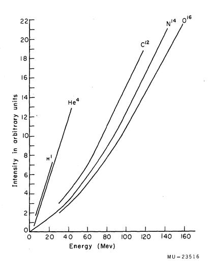
Fig. 8. Response of CsI as a function of energy (from Ref. 16).
