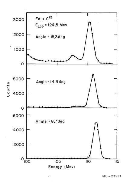
Fig. 11. Typical energy spectra taken with the CsI scintillation counter.
