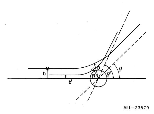
Fig. 1. Classical Coulomb trajectories and scattering parameters.
