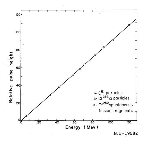
Fig. 10. Response of the solid-state radiation detector to different particles at various energies (from Ref. 17).
