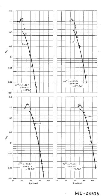
Fig. 24. Rainbow model fits for C<sup>12</sup> elastically scattered from Ni, Ag<sup>107</sup>, In, and Ta (from Ref. 43).
