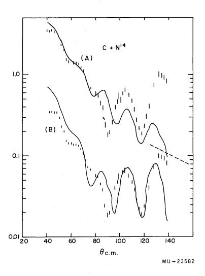
Fig. 29. (A) Same as 25A for N<sup>14</sup> scattered from C. The parameters are  $V_0 = -48$ ,  $W_0 = -5.75$ ,  $R = 1.275A^{1/3}$ , d = 0.575.
