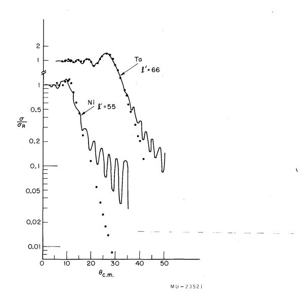
Fig. 3. The differential cross section divided by the Rutherford cross section as a function of the center-of-mass angle (in degrees) is plotted for  $C^{12}$  elastically scattered from Ta and Ni. The dots are the experimental values and the solid line is the Blair sharp-cutoff calculation.
