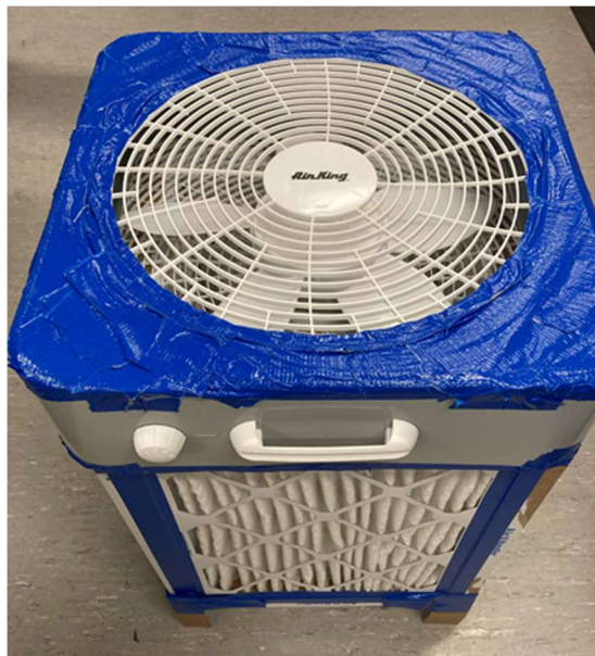
Figure S2-2. A photo of the assembled Corsi-Rosenthal Box.
