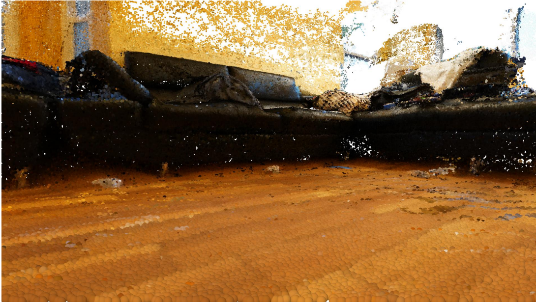
Figure 5.17. Point cloud-based 3D map generated using SLAM on BeagleRover.
