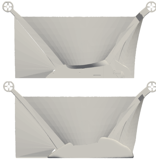
Figure 4.12. The complex mesh body is on top, while the simplified mesh is on the bottom.
