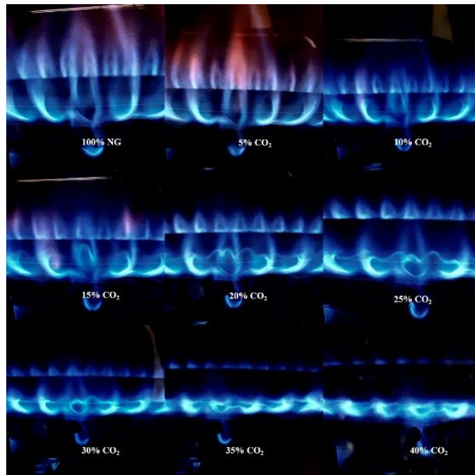
Figure 12. Flame shape for conventional water heater with increasing CO 2 content
