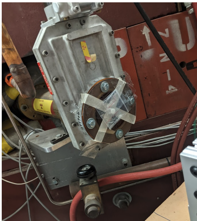
Figure 6.1: In-beam target location. Target was attached to the Mylar face of the beampipe between the cyclotron vault and Cave 5. Figure is looking downstream. Collimator is visible on lower right hand corner. The out-of-beam target is not visible.
