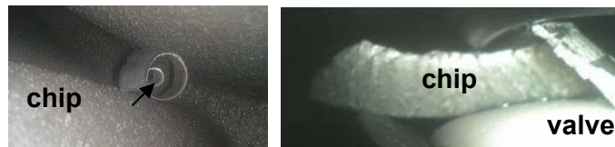
Figure 1.7: Milling chip lodged in a water jacket passageway and an oil valve.
