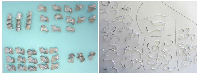
Figure 3.6: Drilling and milling chips sorted by size and shape.
