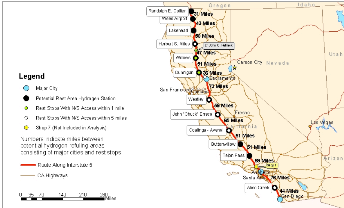
Figure 9 Completed map of proposed stations. All large black dots represent a proposed station. Some black dots have smaller dots inside. This is to indicate additional information indicated in the legend. Note – Distances between stations will likely be smaller near the major metropolitan areas of Sacramento, Stockton, Los Angeles and San Diego. Blue dots indicate city centers and do not represent the extent of suburban development.
