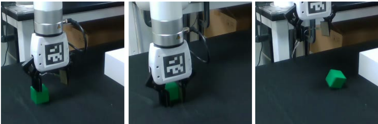
Figure 4.13. Examples of failure modes including cube collisions, table collisions, or permanently dropping the cube.
