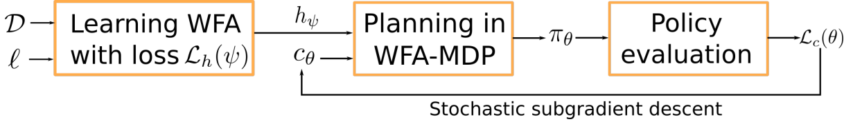
Figure 3.20. WFA-IRL architecture for joint learning of a task specification h_\psi and cost function c_\theta . Given demonstrations \mathcal{D} and a labeling function \ell , we learn the unknown task specification with a weighted finite automaton. We construct a product WFA-MDP space from the learned WFA \psi = \{\alpha_0, \beta, \{\mathbf{W}_\sigma\}_{\sigma \in \Sigma}\} to solve a deterministic shortest path problem with cost estimate c_\theta . The agent policy \pi_\theta is compared with the demonstrated controls to backpropagate the loss \mathcal{L}_c(\theta) with respect to \theta .
