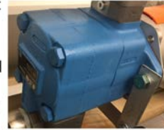
Figure 3.3.3.6: Hydraulic pump for varnish test system.
