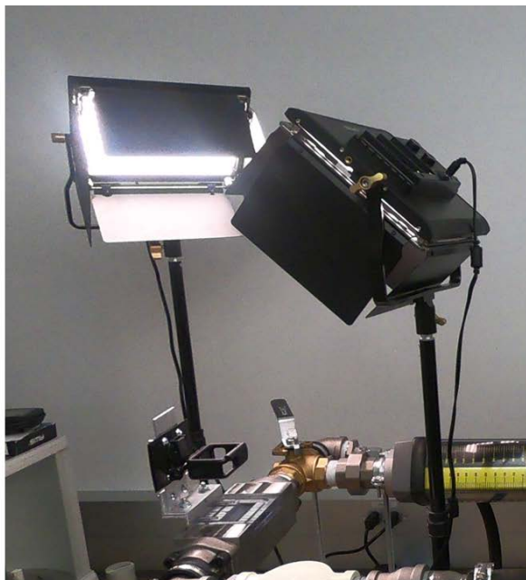
Figure 4.3.2.1: Test cell shown with Neewer NL-660 lighting
