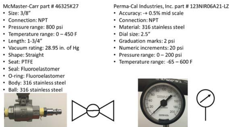
Figure 3.3.11.3: Left: 2 way ball valve. Right: pressure gauge.
