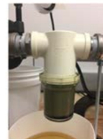
Figure 3.3.9.1: Filter for varnish test system.
