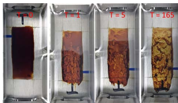
Figure 5.3.1.2: Test 2 showing the movement of varnish on the coupon at 0, 1, 5, and 165 minutes. The test cell lid was removed and the coupon was imaged in the test cell while covered in fluid.
