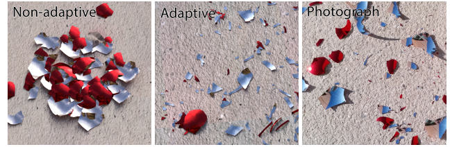
Figure 10: The shattering of a spherical glass ornament is simulated using our adaptive algorithm (middle), and a statically meshed version with the same triangle count (left). The fracture pattern of the adaptive simulation is similar to an actual experiment (right), while the simulation without remeshing fails to correctly resolve the fracture dynamics and produces an unrealistic distribution of shards.
