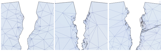
Figure 5: In this example, we tear a sheet with our algorithm (left) and the separation tensor of O’Brien and Hodgins [1999] with fracture substepping (middle) and without substepping (right). Our algorithm produces significantly fewer artifacts in simulations with varying triangle size.
