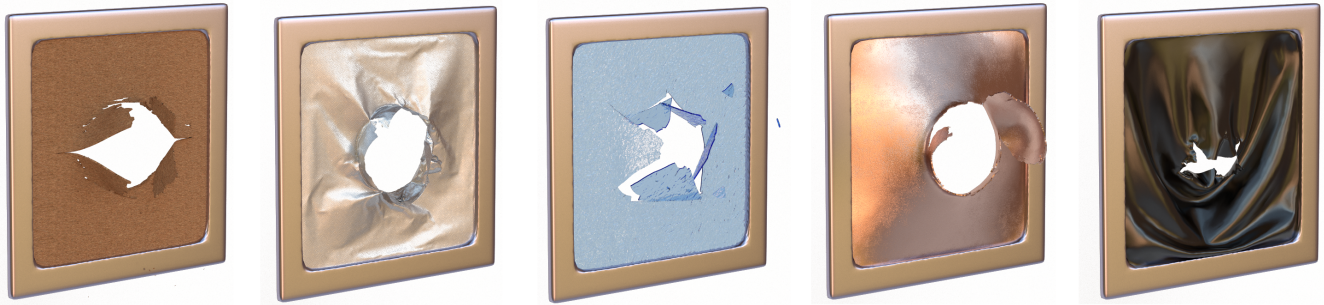
Figure 1: Our method produces realistic tearing and cracking phenomena for thin sheets made from a wide variety of materials such as cork, foil, plastic, metal, or vinyl. These results are achieved using simulation on adaptive meshes that resolve fracture behavior at very high resolution.
