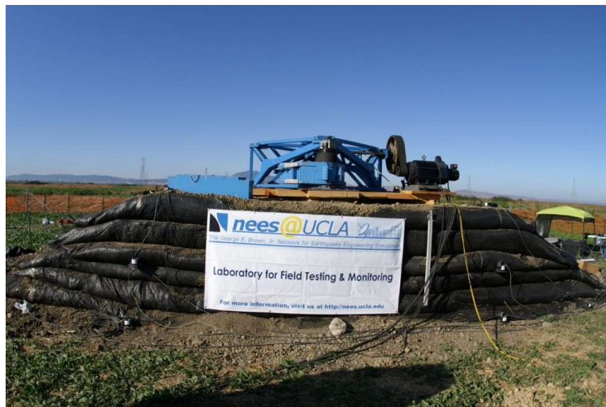
Figure 4. MK-15 eccentric mass shaker mounted atop test specimen.
