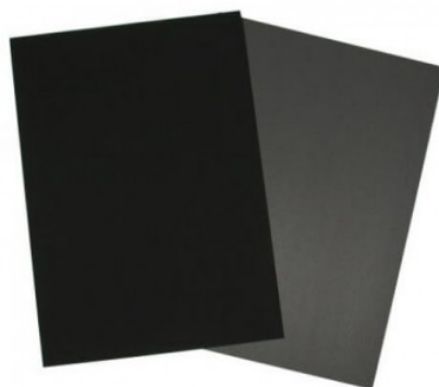
Figure 1.5: Carbon fiber paper (dark side represents MPL, gray side represents the bare side with no MPL [30]).
