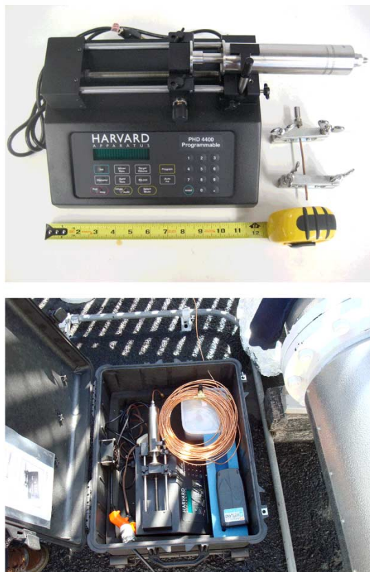
Figure 1. (top) The Harvard syringe pump apparatus with stainless steel syringe along with sectioned Cu tubing of 12.7 cm (5") length. Note the sectioned Cu coil with two refrigeration clamps and ultratorr fitting attached to one end. (bottom) Deployment of SPARTAH at the San Bernardino wellhead. The Pelican case houses the syringe pump apparatus and one Cu coil. One end of the coil is attached to the syringe, and the other leads through a hole in the case to the wellhead.
