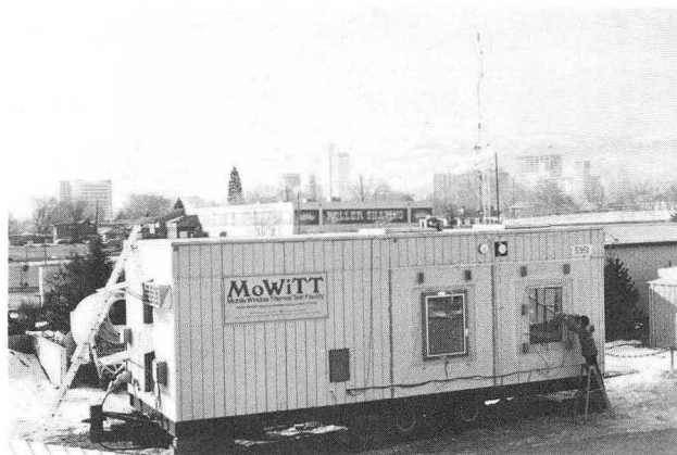
Figure 8. The MoWiTT facility at its field test site in Reno, Nevada. Two sealed insulating glass units are mounted in the two calorimeters. Portable building at left contains computer that controls the facility and records data, including data from on-site weather tower. (CBB 892-812)
